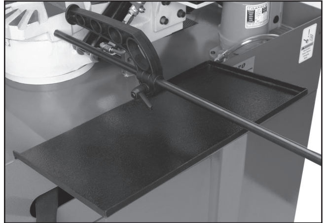
Figure 20. Splash tray installation.
